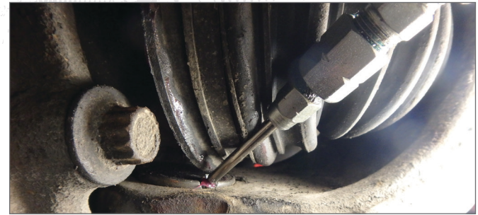
In applications with tight clearances, low-profile zerk fittings make injecting fresh grease easy and possible.
